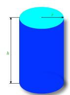
$Volume_{prism} = Area of Base \times Height, (Remember, a cylinder IS a prism)$
