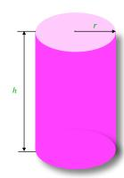
Surface Area =  $2 \times$  Area of Circle + Area of Rectangle  $= 2 \times \pi r^2 + \text{Lenght} \times \text{Width},$  $= 2\pi r^2 + 2\pi r \times h.$
